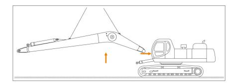
4.2.2. Install and secure the boom on the machine by means of the bolt.
