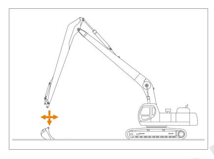
**4.2.12.** The Long Reach arm has a far longer reach than a standard arm. As a result, it is necessary to reduce the oil flow in the bucket closing cylinder. If you do not reduce the oil flow in the cylinder, this may decrease the level of the bucket (closing / opening) movement precision and it may lead to a damage of the bucket.
