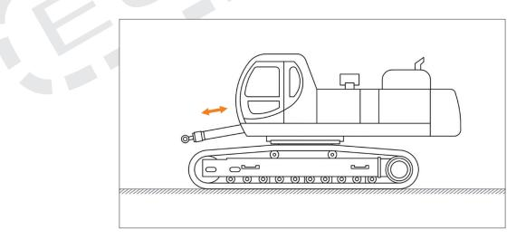
4.1.3. After removing the genuine arm, leave two cylinders raising the arm immediately next to the machine.
