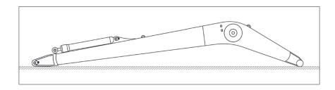
**4.1.7.** Transfer the arm fold cylinder from the standard arm to the Long Reach arm. Check if it has been properly installed. Connect and properly secure the hydraulic hoses.
