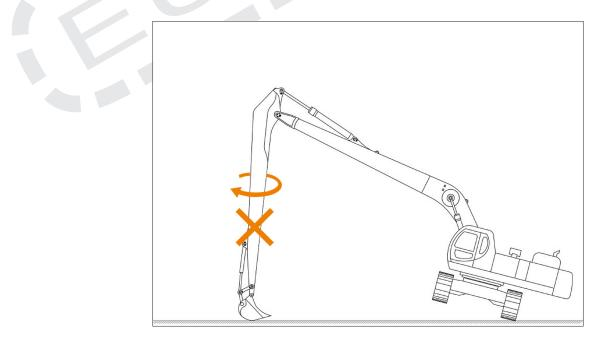
С Є 6 **1.3.4.** Never use a excavator equipped with the Long Reach arm for carrying out works for which a crane has been designed.
