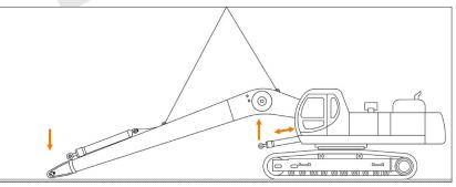
4.2.5. Connect and safely attach all hydraulic hoses connecting the machine to the Long Reach arm as well as those provided at the end of the arm.
